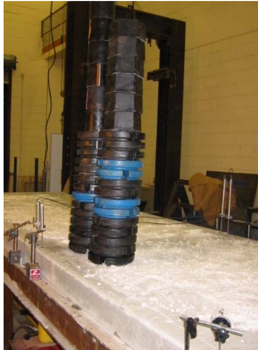
Figure 10. Slab 2 being jacked up at a corner with 400 kg concentrated load applied to adjoining slab.
