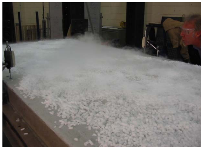
Figure 3. Dry ice was uniformly distributed on concrete slabs
