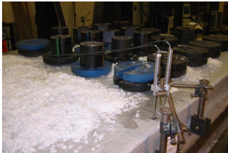
Figure 6. 400 kg dead load added on the Slab 1
