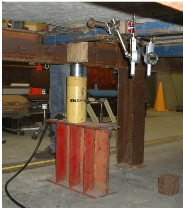
Figure 6. Slab 1 being pushed up at a corner
