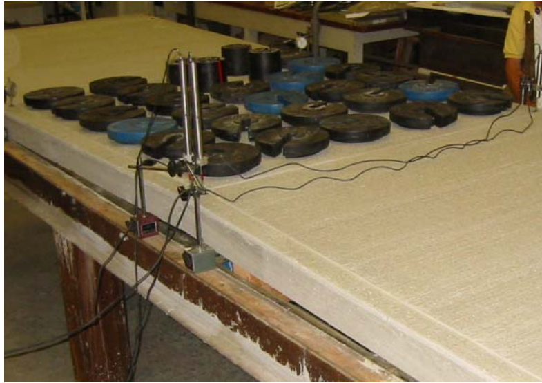
Figure 5. 300 kg dead load added on the Slab 2
