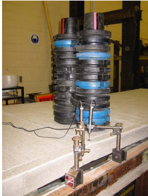
Figure 9. Slab 1 being jacked up at a corner with 300 kg concentrated load applied to adjoining slab
