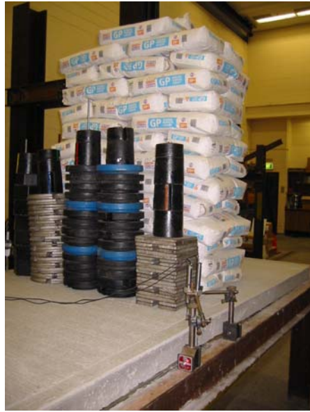
Figure 15. Slab 2 being jacked up at line EF with 2,000kg load added on Slab 3
