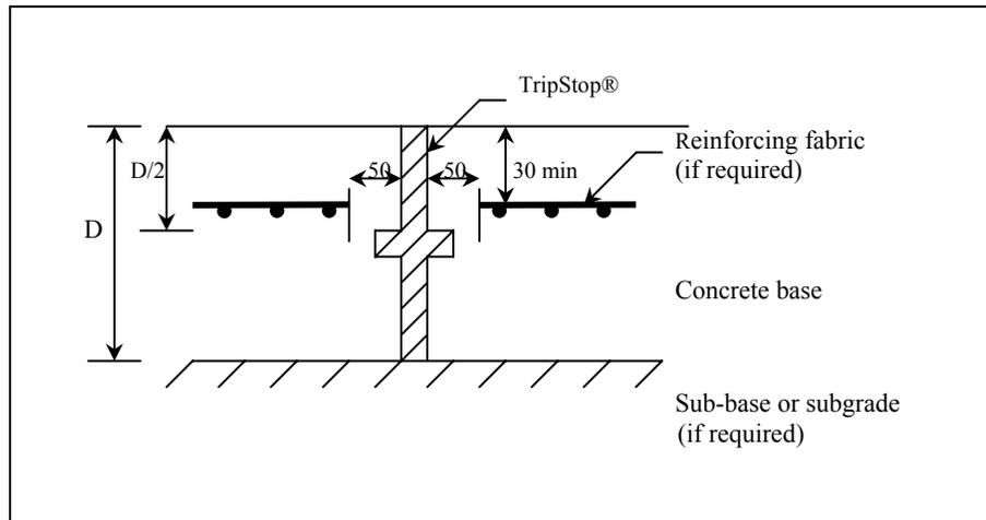
**Figure 4: TripStop® joint**
