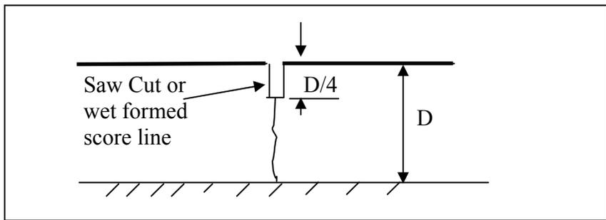
**Figure 1: Control joint in an un-reinforced footpath slab**
