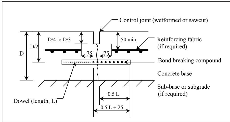
**Figure 3: Dowelled Control Joint<sup>2</sup>**
