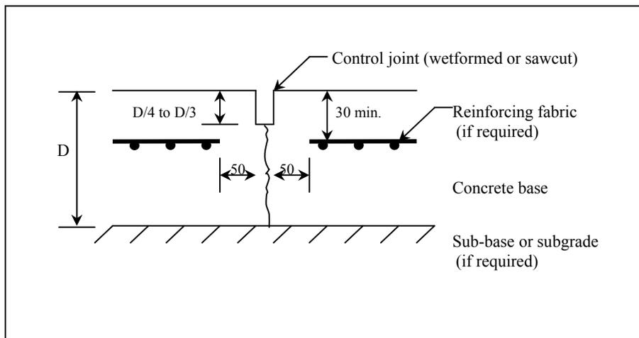
**Figure 2: Control joint in a reinforced footpath slab**
